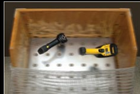
Loose Cargo Stress Test - 10 Hours of Random Tumbles Against Metal Surface
