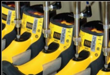
Trigger Test - Tested to 10 Million Cycles
